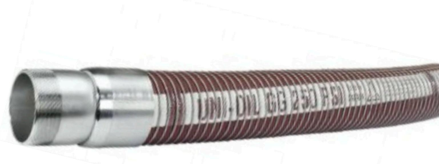
THE UNI-OIL<sup>™</sup> GG IS DESIGNED FOR THE TRANSFER OF A WIDE RANGE OF PETROLEUM PRODUCTS AND ARE IDEAL FOR THE TRANSFER OF MEDIA FROM STORAGE TANKS AND PROCESS PIPING TO RAIL CARS OR TANK TRUCKS. MULTIPLE PLIES OF POLYPROPYLENE FILMS AND FABRICS ARE ENCASED IN A POLYESTER VAPOR BARRIER FOR SUPERIOR OPERATION.
