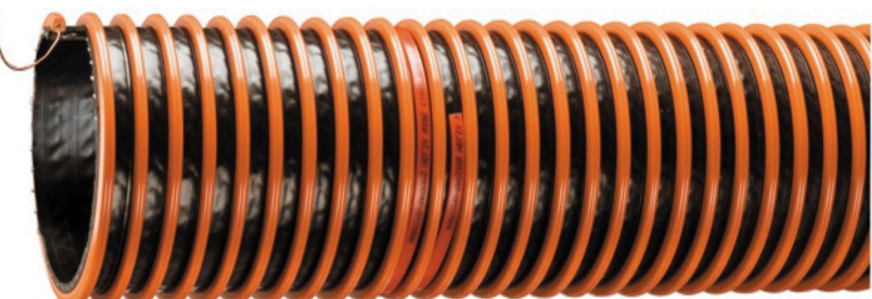
Construction: Specially blended nitrile (NBR) rubber tube with polyester fabric reinforcement, rigid PVC helix and embedded grounding wire.
